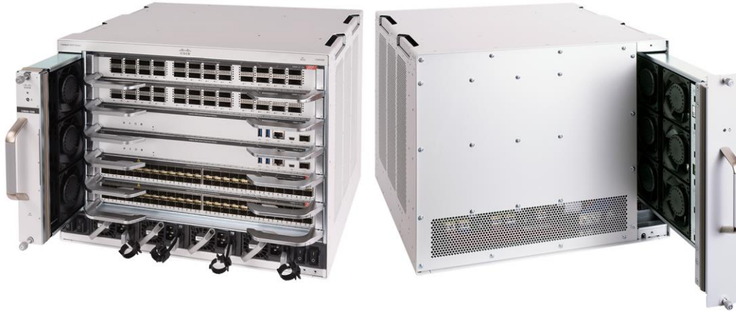
Figure 2. Cisco Catalyst 9606R Chassis with Fan Tray
